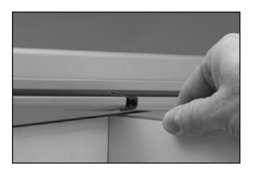
Hinges have to be mounted when the lockers are in upright position. In the accessories you will find a template.
