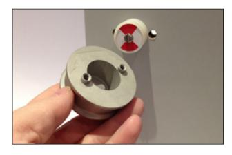
Insert the groundpart (POM) from the other side and fix it through the lock housing with the indicator part with 2 screws M5 x 45 (Torx 20) .
