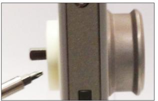
Fit the turned part on the ground part (POM). Hole for the setscrew has to point downwards. Now fix it with 2,5 mm allen key.
