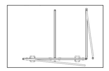
The corner profile is placed on the top of the side wall panel.
