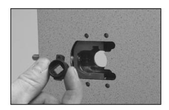
Assemble groundplate with small notch (for red/white outside), stainless steel plate and screw
