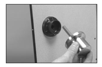
Fit red/white indicator on the square at 11 o`clock position with the door opened (latch slided-in). Fix the red/white ground part with setscrew M5 (allen key 4) on the square.
