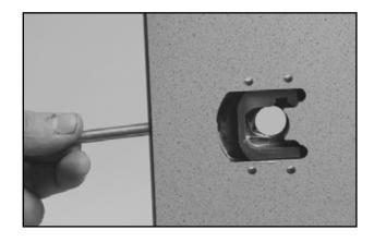
Fix the rounded bolt at the slider by lock ring
